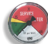
MC-12 RETURN LINE INDICATING GAUGE FOR 15 PSI FILTER APPLICATIONS 2" MULTICOLOR 0-12 PSI GREEN 12-15 PSI YELLOW 15-60 PSI RED (SERVICE FILTER)
